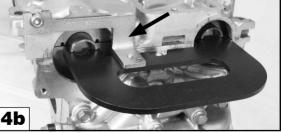
Construct the Camshaft Setting Plate Assembly by using the AST4561 Plate and attaching to it the appropriate Location Bracket – The Rightangled Bracket shown in **4A**, or the Extended Bracket – shown in **4B**.
